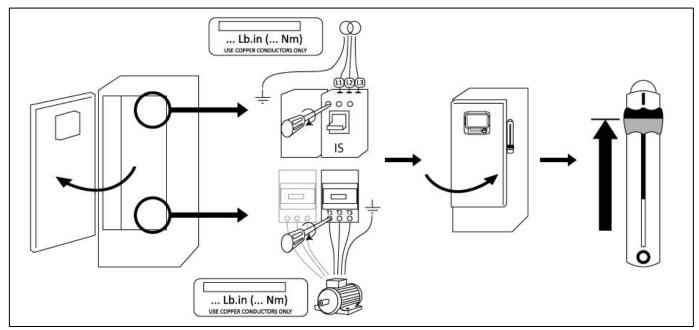
Connect the input power and the motor on their respective terminals. Secure with the appropriate torque as indicated on the torque label and verify all connections.
