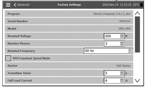
This page is used to visualize the program version, the serial number and the model of the controller.
