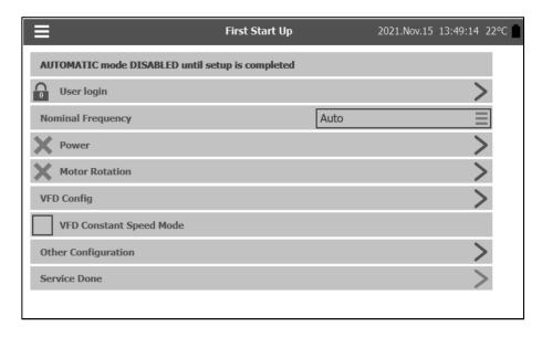
Once the VFD parameters has been verify and the Autotune has been performed, continue with the "First Start Up" page. The controller will automatically detect and display the frequency of the power source. It is then possible to manually choose the frequency of the voltage.
