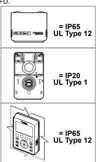
It is possible to remove the Graphic Display Terminal and to place it on the enclosure door using the door mounting kit. The UL IP is Type 12 if the door mounting kit is in the closed position without the Graphic Display Terminal or if the Graphic Display Terminal is installed. If the door mounting kit is in the open position without the Graphic Display Terminal, the UL IP is Type 1.
