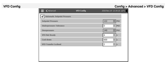
This page is to modify and to vision parameters specifics to the usage of the VFD.
