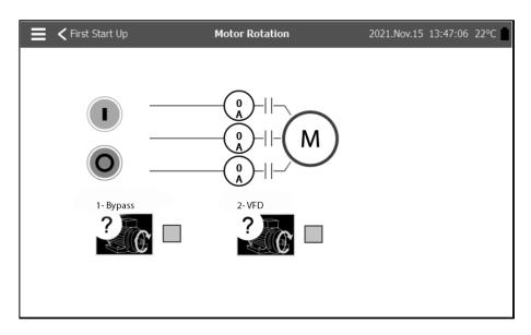
Place VFD mode switch in BYPASS mode.
