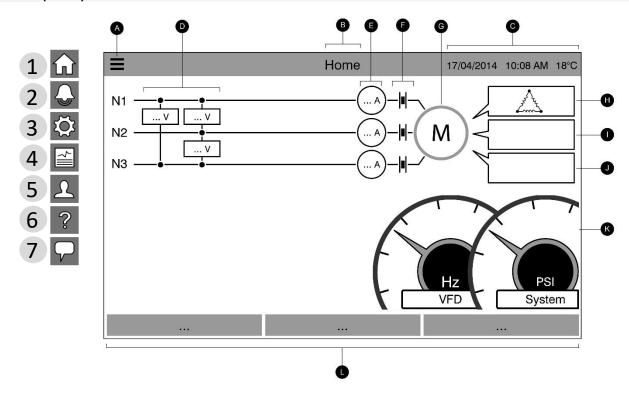
The home page displays all controller statuses and important values of the controller. This includes all voltages, currents, pressures, motor state and status, as well as all timers and motor starting sequences.
