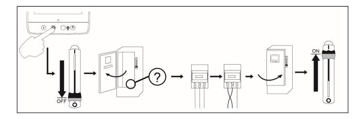
Place VFD mode switch in VFD mode.
