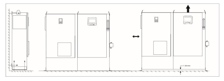
Verify that the controller is installed securely on the wall, or on the mounting stand.
