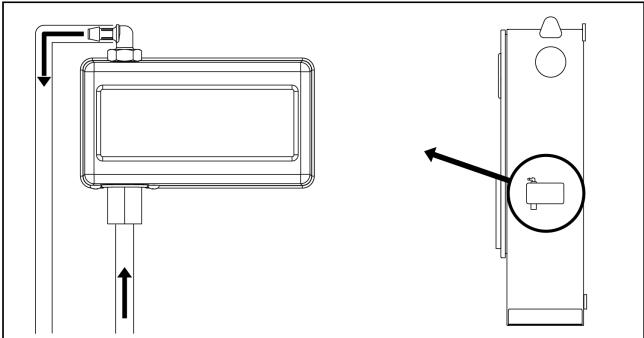
Verify and/or install the proper water connections for the water input and the drain. They must be securely installed and tightened. Refer to the silkscreen markings on the plastic cover.
